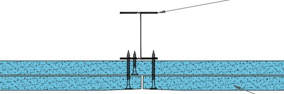
2x15mm Knauf Soundshield Plus fixed with SPEEDLINE Drywall Screws at 300mm centres (200mm centres at external angles). Ref to table for fixing length.
